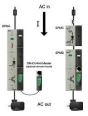
The SPMA solution will be lower cost but the SPMD solution may give site standardization. The master control module on the drive may be replaced by a follower module and the master can be remotely mounted, as the application requires.
